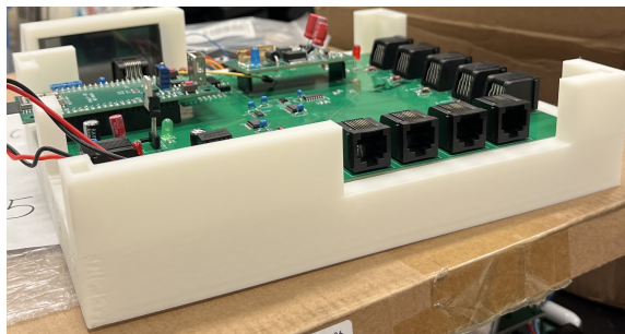
Fig. 8.24: Motherboard Housing (Top Off) with Motherboard Inside
