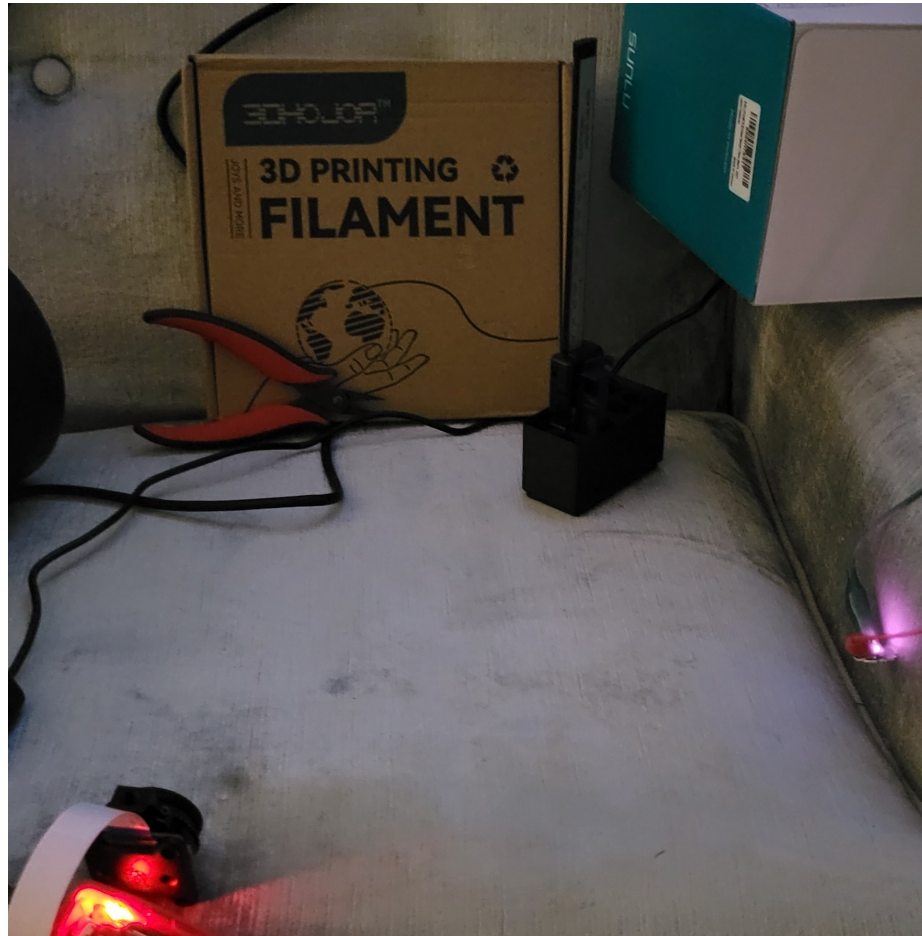
Fig. 9.21: Setup for IR image (captured with cell phone camera, the global shutter camera and custom lens is visible in the bottom left, and an 850 nm IR LED is visible on the right)
