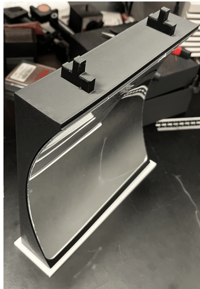
Fig. 8.17: Parabolic Mirror Mount with Mirror Attached
