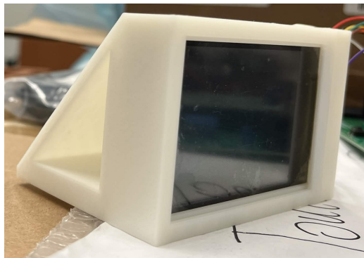
Fig. 8.26: Waveshare Screen Mount with Screen Inside
