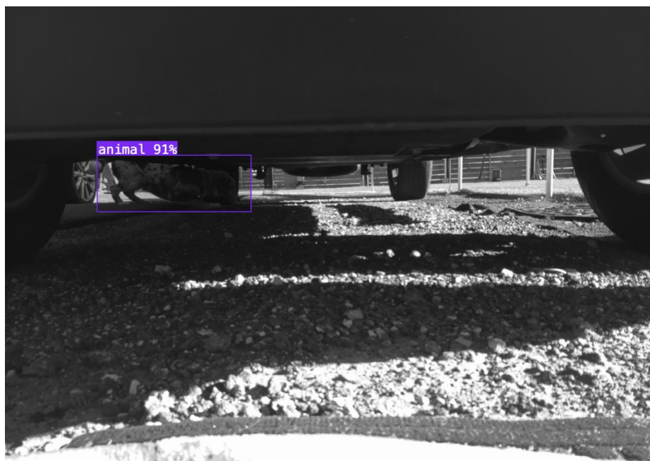
Figure 9.3.2 Detection output showing identified animal beneath the vehicle with confidence score
