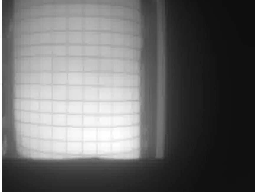
Figure 4. Laboratory near-infrared image capture of a physical calibration grid (1.0 in. horizontal by 0.5 in. vertical spacing) utilized to verify uniform horizontal compression and spatial resolution across the active field.
