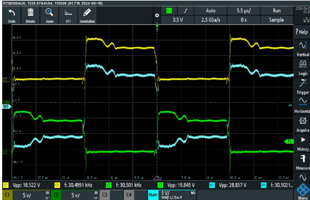
Figure 5. Ultrasonic alarm characterization: amplified 12 V output at 30.5 kHz.
