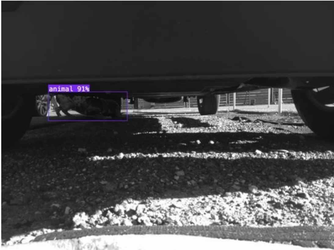
Figure 6. YOLOv11 detection outputs on under-vehicle imagery showing localized animal detections with confidence scores.
