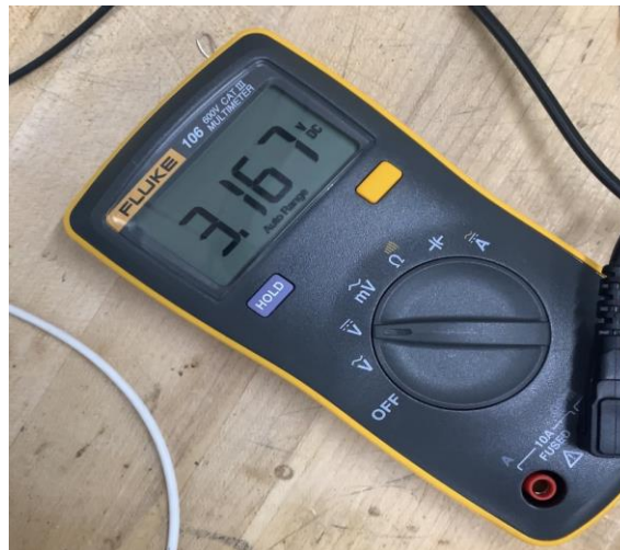
Figure 9.13: 3.3V General Regulator Output Under Load
