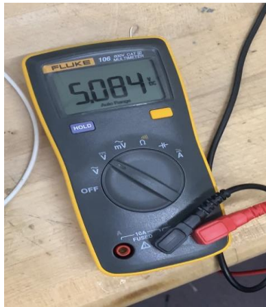
Figure 9.12: 5V Regulator Output Under Load
