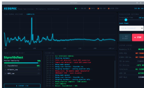
Fig. 4. ECOSpec user interface displaying real-time Raman spectrum acquisition, system status, and results.
