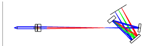
Fig. 3. First-order ray trace of collection optics, starting at the sample scattering on the left.
