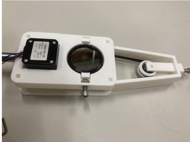
Fig. 4. Custom belt driven quarter waveplate rotator
