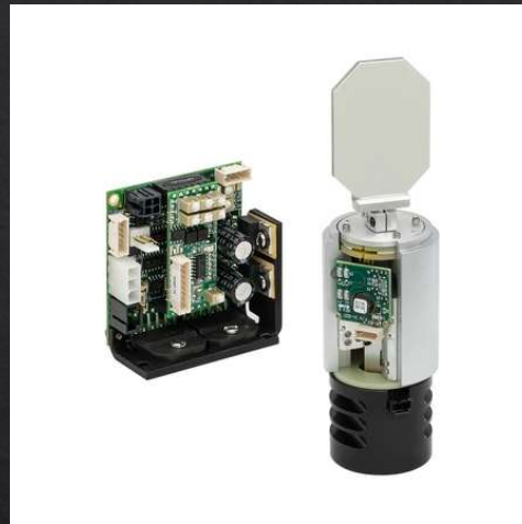
Single Axis Cross-Flexure Galvo Motor, from ThorLabs
