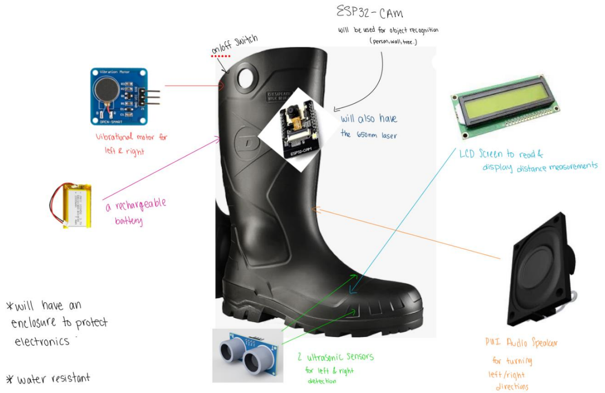
Figure 6: Initial Prototype Design with all components
