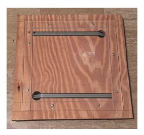
Figure 9.4 Top View: w/ Force Sensitive Resistors (FSR) placed under acrylic tile
