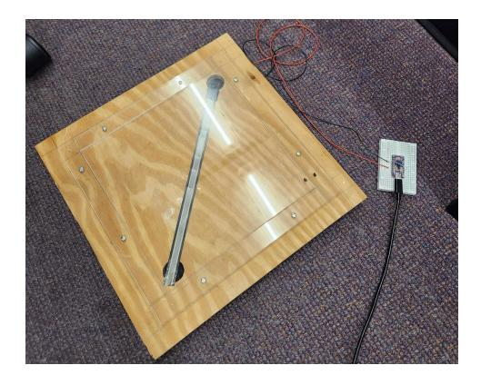
Figure 9.6 Mini demo video pad with breadboard and single FSR integration
