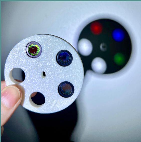
3D printed optical filter wheel with chosen filters.
