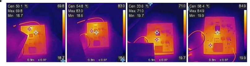
3.3V Regulator @ 69.8°C. To: -40°C ≤ Tj ≤ 150°C. 3.3V Diode @ 83.0°C. To: -55°C ≤ Tj ≤ 150°C 5V Regulator @ 71.0°C. To: -40°C  $\leq$  Tj  $\leq$  150°C.
