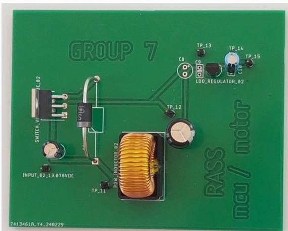
Fig. 2. Power supply unit for MCU and servo motor
