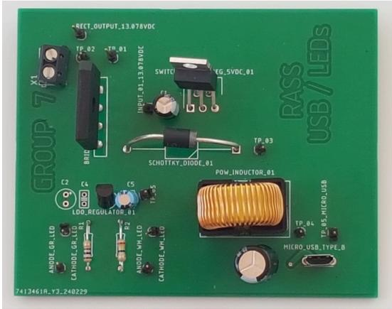
Fig. 1. Power supply unit for micro-USB and LEDs
