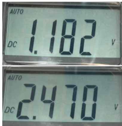
Figure 76: Voltage Across First Resistor, Low Power (top), High Power (bottom)
