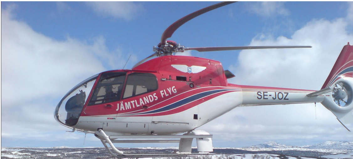
Figure 33: Rolling Shutter Distortion
