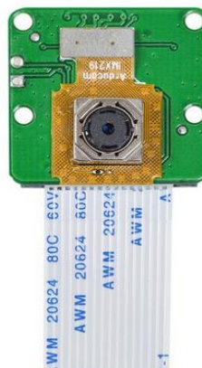
Figure 37: Arducam NoIR IMX219-AF Programmable/Auto Focus IR Sensitive Camera Module for Nvidia Jetson Nano
