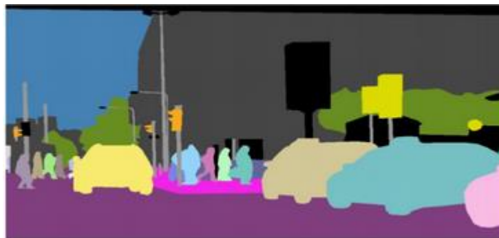
Figure 63: Panoptic Segmentation including the instance and semantic segmentation
