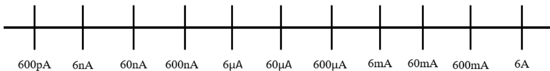
Figure 30: Decade divisions of photocurrent for responsivity of 0.6\text{A/W}
