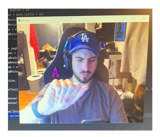
Much of our application testing took place during preparation for the midterm demo video. To test our gesture detection accuracy specification, we flashed each sound generating gesture onto the screen 10 times, and recorded whether or not the proper tone was output. Below is a table summarizing the 10 runs. Our average detection accuracy was 95.71%, which meets our specification of 80% or better.
