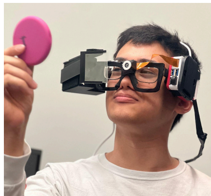
Figure 7: One of the colleagues testing the glasses' color detection values.
