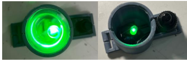
Fig. 12. A side-by-side view of the collar tag turned on with the Fresnel lens (left) and housing the electrical components (right).
