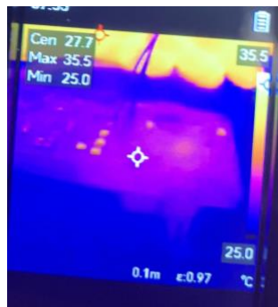
Fig. 14. Picture of the heat dissipation issues the board had.
