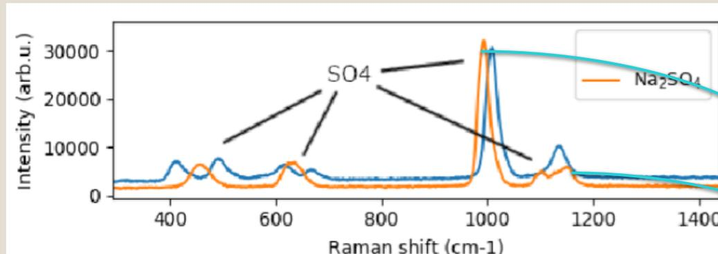
Raman spectrum of Sodium Sulfate. Image taken from <https://www.researchgate.net/figure/Example-Raman-spectra-of-CaSO-4-and-Na-2-SO-4-Both-show-typical-sulphate-Raman-modes>
