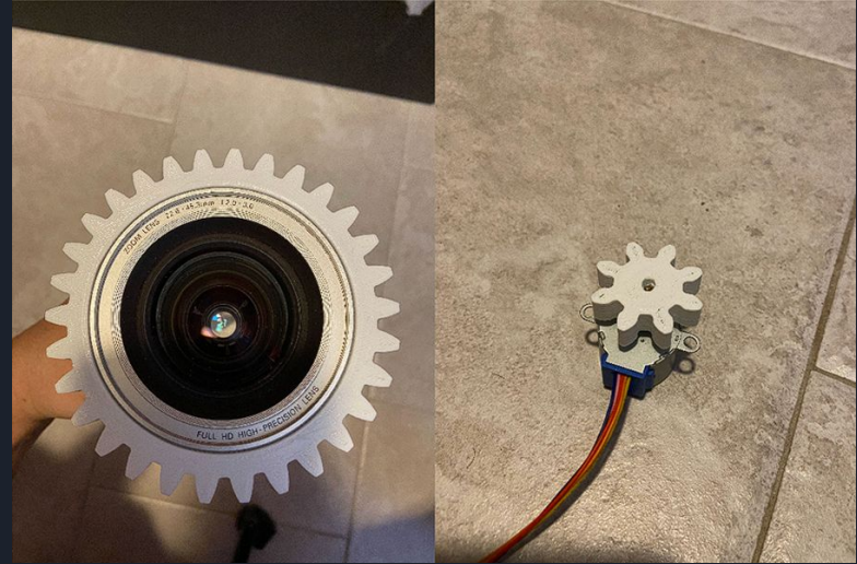
Gear system integrated onto motor and projection lens
