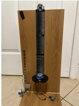
Fig. 10. 3D printed microscope body assembled with the stage and turntable on wooden platform
