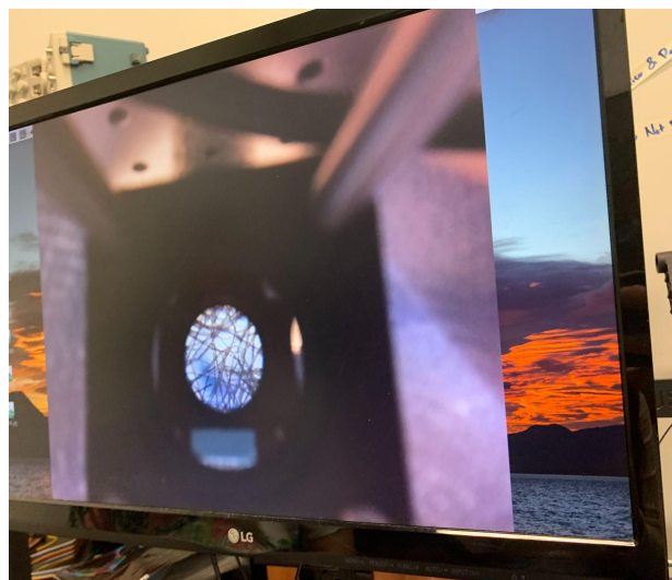
Figure 7.0.5 Tissue paper sample with white LEDs
