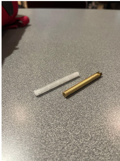
Figure 4.8.2-2. 3D Printed Side Loaded Fiber Chuck
