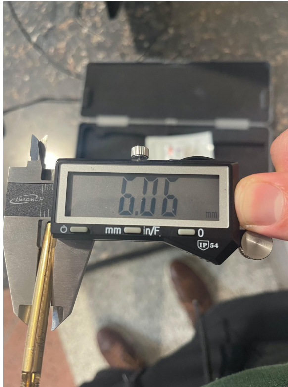
Figure 6.1.2 Chuck diameter, needed to fit printed chuck into chuck holder.
