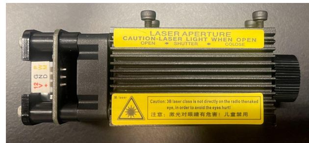
Fig. ###. Laser used in Optical Engraving Process
