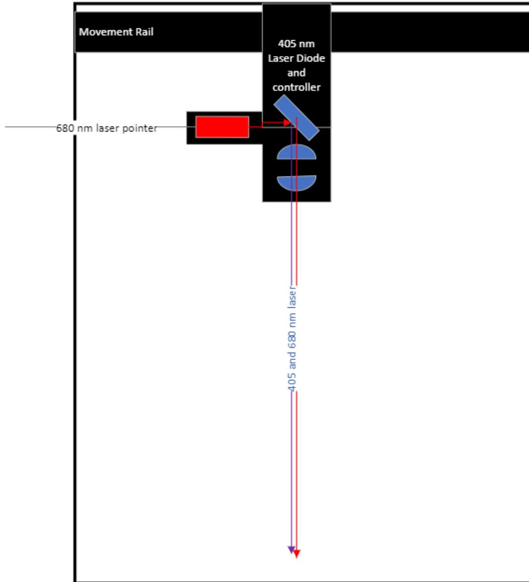
Figure 23; Optical Workspace Detection System mounting option 2
