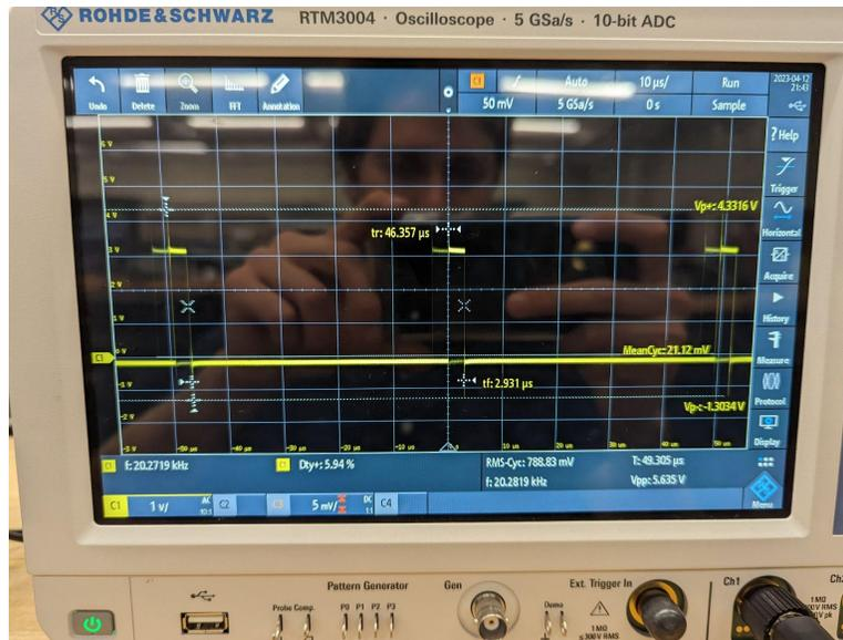
Figure 65; Oscilloscope output from laser controller of a 20 kHz 6% duty cycle PWM signal
