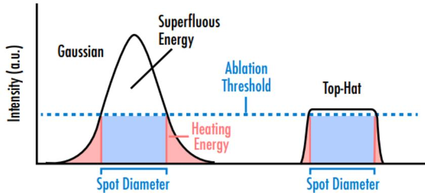
Figure 7-8; Gaussian, Flat Top, and Top-Hat beam profiles[1]
