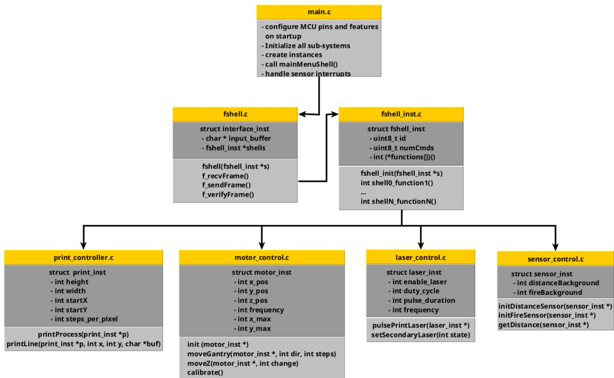
Figure 36; General firmware components and program flow
