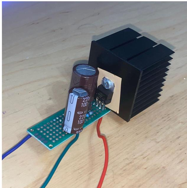
*Figure 40; LM317 Adjustable Regulator prototype with 12V output*
