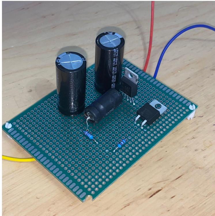
*Figure 41; LM2576 Adjustable regulator with 12V output*
