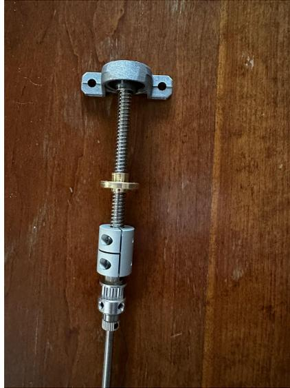
*Figure 69; Threaded rod with pulley assembly*
