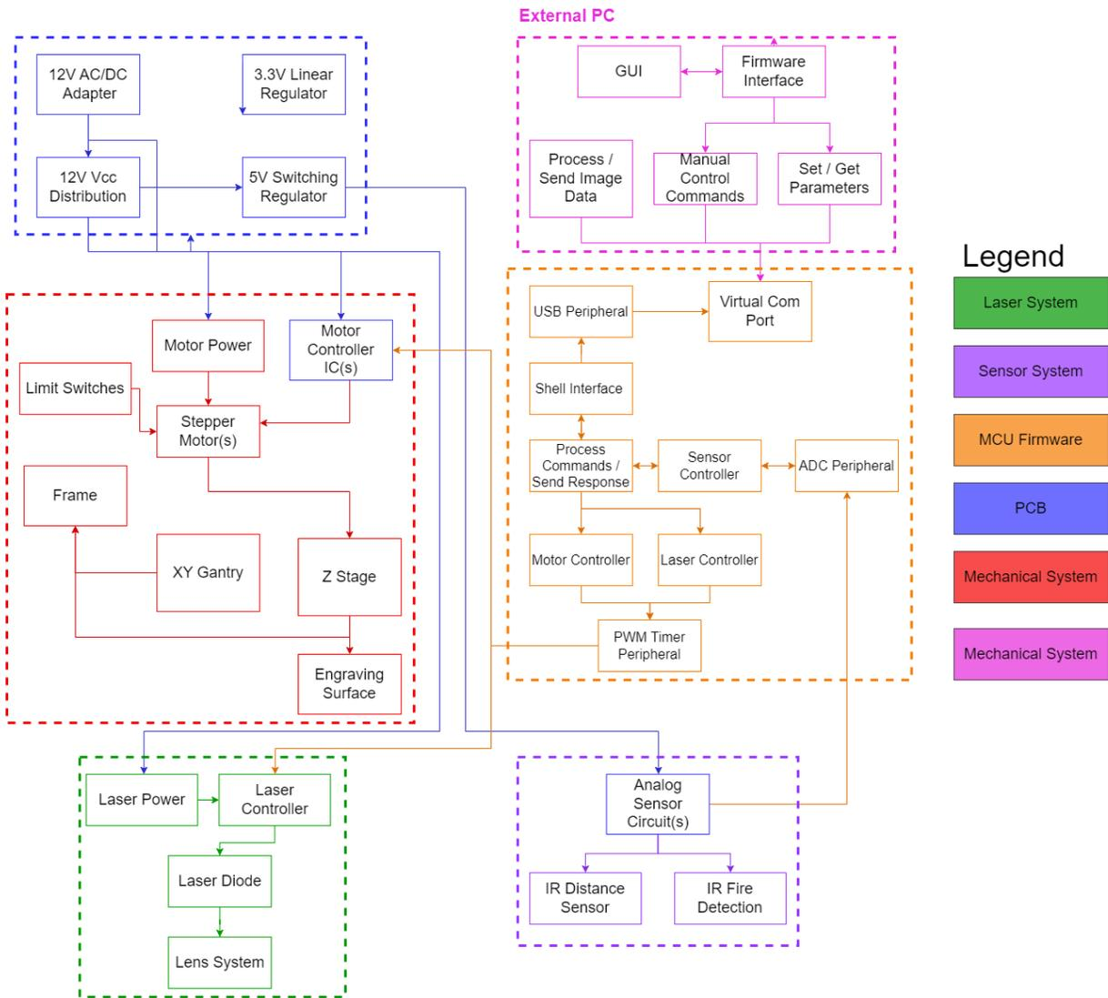
Figure 3; Subsystem block diagram and distribution of work
