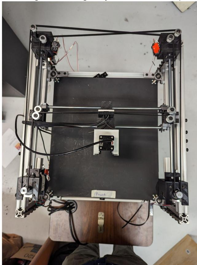
*Figure 68; Final XY gantry version mounted to frame*
