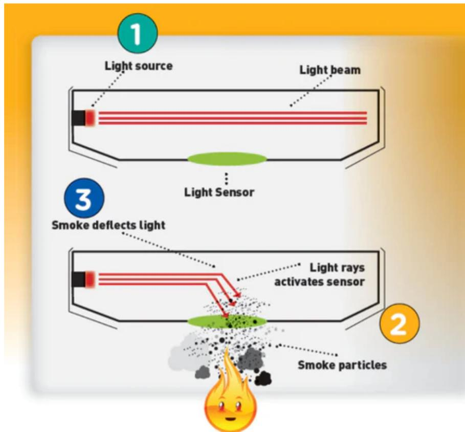
Figure 10; How an optical fire alarm works[19]
