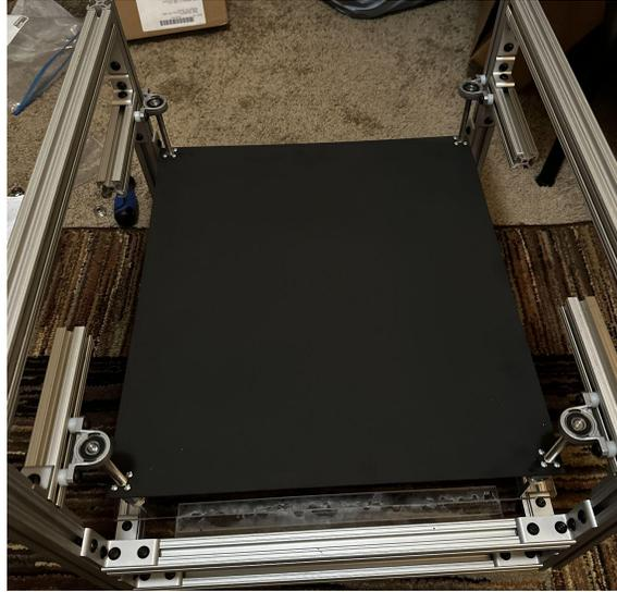
*Figure 71; Z-stage of D-MILE with print bed*
