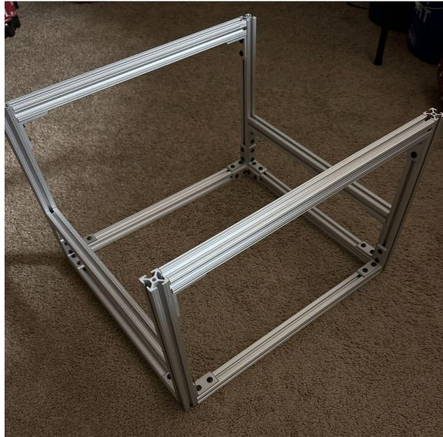
*Figure 66; Frame of D-MILE before any components*
