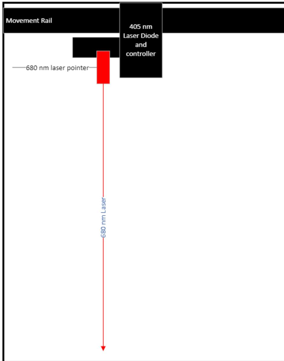
*Figure 22, Optical Workspace Detection System mounting option 1*
