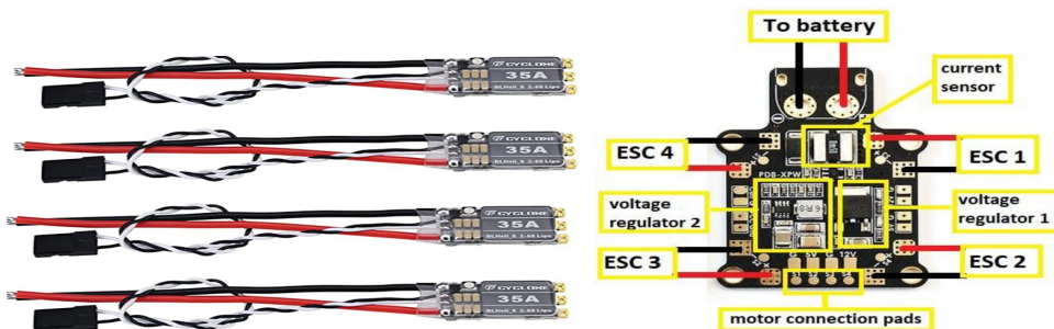
Figure 3.13.2: Electric speed controller for brushless motors and the power distribution board
