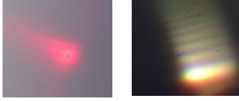
Fig. 3. Output of the etalon with (left) a 633 nm laser input and (right) the collimated LED input, utilizing a focusing lens for detection.
