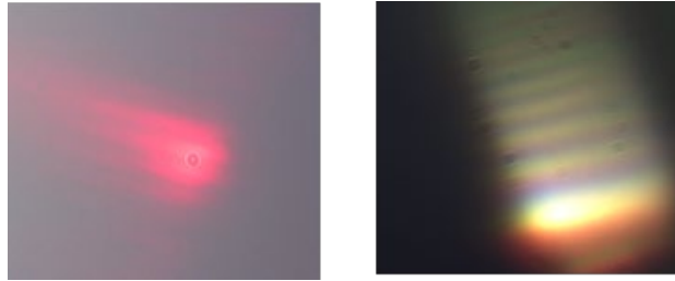
Figure 9.1.2.1 Etalon outputs from (left) red aligned HeNe beam and (right) the collimated LED, utilizing a focusing lens for detection.
