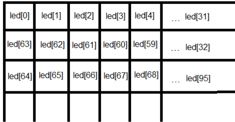
Figure 18: LED Addressing Scheme Using Snaking LED Strand
