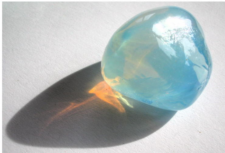
Figure 24: Example of Rayleigh scattering where it can be seen the shorter wavelengths (bluish) are scattered in the glass and the longer wavelengths (reddish) are transmitted [41]. Image used under creative commons.
