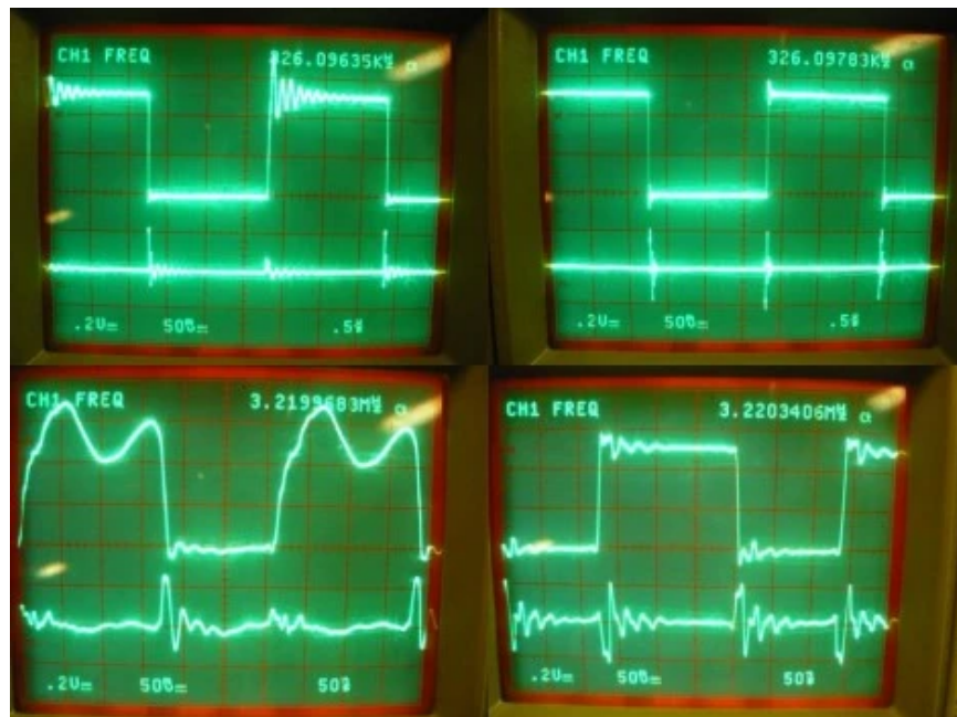
Figure 49: Two Different Inverter Signals, Displaying the Difference Between Decoupled and Not Decoupled Signals. From left to right and top to bottom, the signals are: Signal one untreated, signal one decoupled, signal two untreated, signal two decoupled. Image used from Hackaday.com [119].
