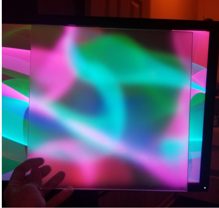
Figure 26: Light diffuser panel softening a complex LED dense display image. Image provided by Lazer Pong project team.
