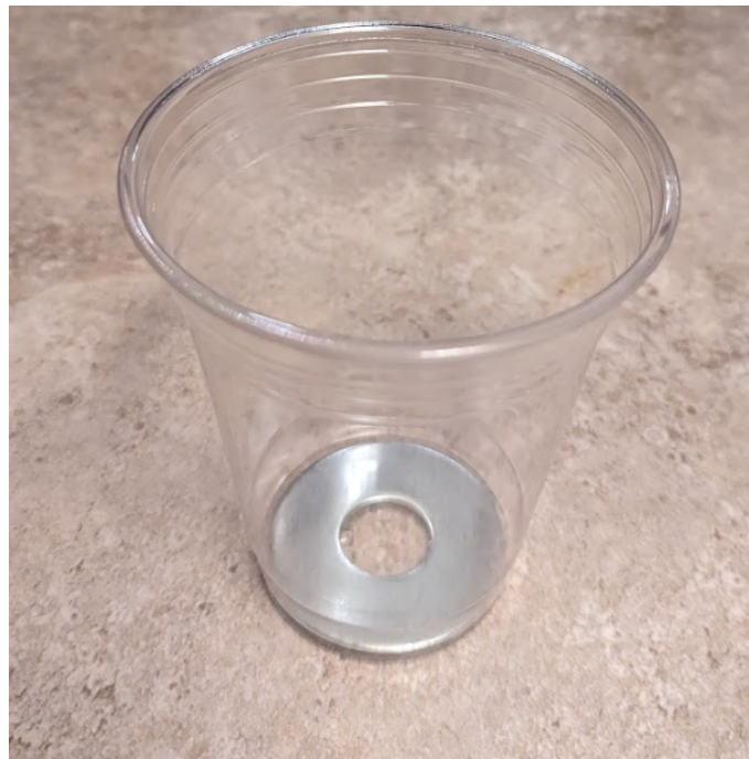
Figure 9: Clear scoring cup with washer weight. Image provided by the Lazer pong project team.
