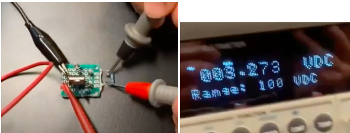
Figure 46. Voltage Regulator Testing
