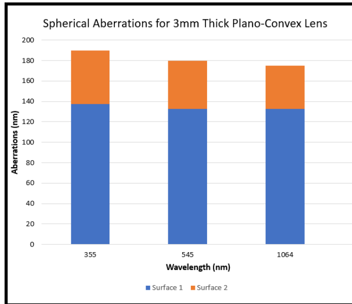
Figure 18: Sum of the spherical aberrations for 355 nm, 545 nm, and 1064 nm. Wavefront error is in units nm and separated by surface 1 and 2 of the lens.
