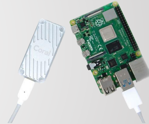
Raspberry Pi 4 + Coral Accelerator
