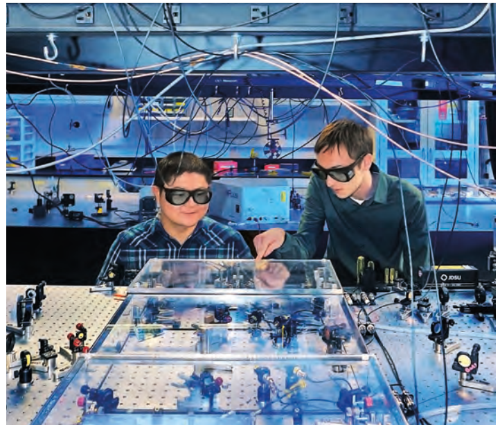
Qitian Ru (l) and Zach Loparo perform spectroscopic experiments with mid-infrared frequency combs.
