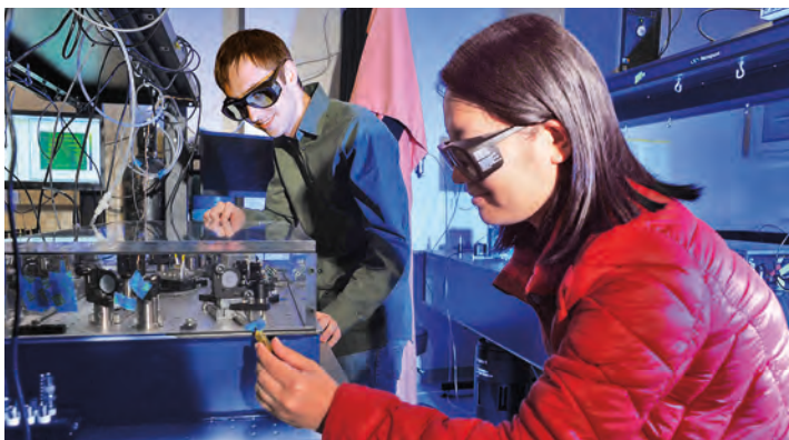
Zach Loparo (l) and Suyuan Chen build a broadband mid-infrared optical parametric oscillator for spectroscopic measurements
