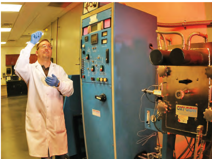
Graduate student Matt Julian is inspecting a transparent laser ceramic after vacuum sintering.
