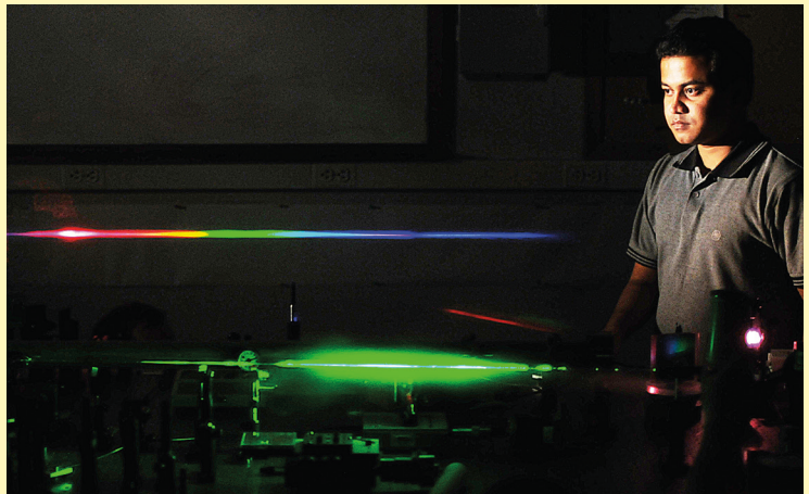
Demonstration of white light continuum generated by high power laser.
