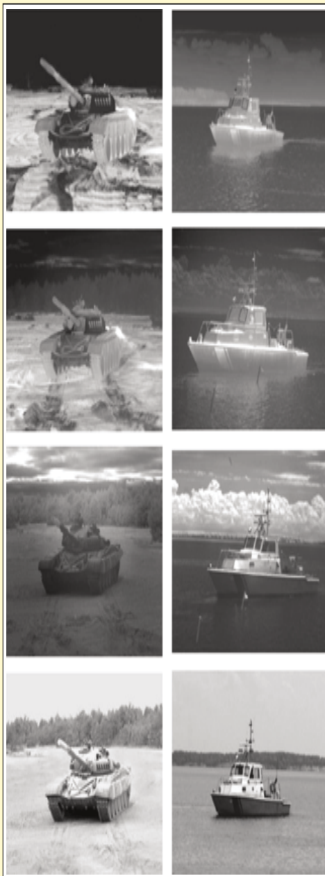
Images acquired at different bands can be very different. Bottom tank and boat are VNIR (0.4-1 μm), next up SWIR (1-1.7 μm), third up MWIR (3-5 μm), top is LWIR (8-12 μm).
