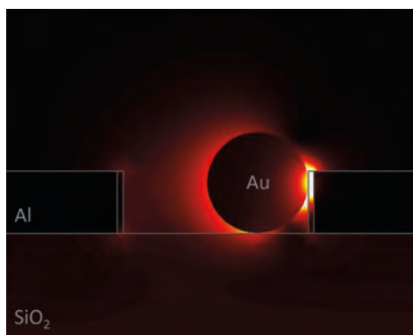
Fig. 3: side view of the simulated gap plasmon enhanced field enhancement
