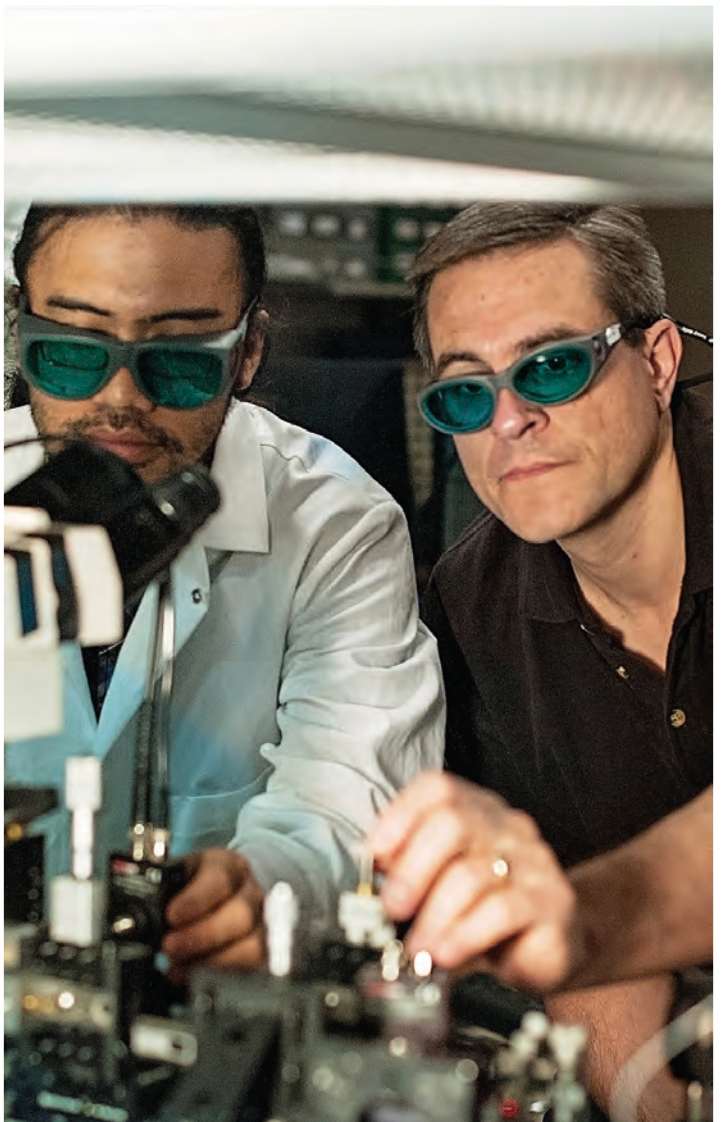
CREOL student Jennefir Digaum (L) and Dr. Kuebler characterize 3D-printed nano-photonic devices that can direct light beams through ultra-sharp turns, in areas as small as a white blood cell.
